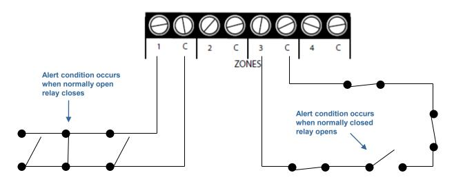
Multiple normally-opened relays wired in parallel (example using Zone 1)
