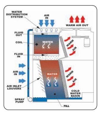
Similarly, in a closed circuit cooling tower or evaporative condenser, the heat is rejected indirectly from a fluid or vapor flowing through the coil section by spraying recirculated water over the coil section, again evaporating a small percentage of the water in the process.
