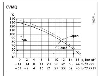
The two curves are shown with the valve's spring setting equal-ling the factory setting. If the spring setting is changed to a higher pressure, the curve will be displaced correspondingly to a higher temperature.
