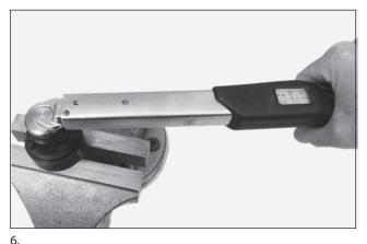
Tighten the washer plate using a torque wrench.
