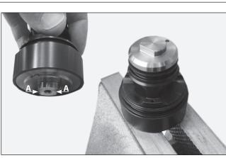
Turn the module upside down and secure in a screw vice, holding the module on the two flat sides (A).
