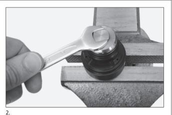
Loosen the washer plate using a 13 mm (0.5 in.) spanner.
