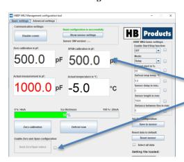
When the sensor is installed and the evaporator is dry and without ice, connect the sensor to the HB-tool using a USB cable.
