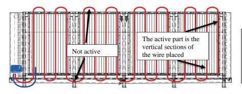
The temperature sensor should be placed were ice melt slowly. Keep away from the hot tubes or electrical elements used for defrosting.
