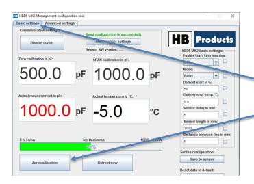
Connect power supply to the box Connect the HB-tool to the box Open basic settings tab Click on the zero-calibration button.
