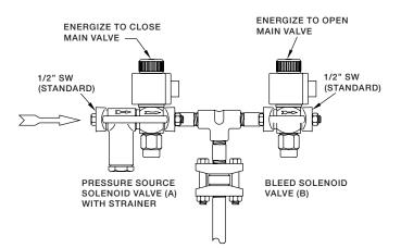
Note: For Pilot Valve Replacement Parts, see Hansen HS6 Solenoid Valve Bulletin S117.
