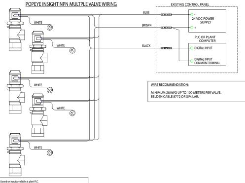
\*Note: Only one signal output can be used at a time. Select PNP or NPN based on inputs available at plant PLC. Consult a controls specialist or PLC manufacturer to determine which input is available.
