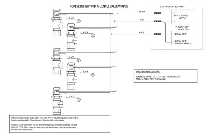
\*Note: Only one signal output can be used at a time. Select PNP or NPN based on inputs available at the plant PLC. Consult a controls specialist or PLC manufacturer to determine which input is available.
