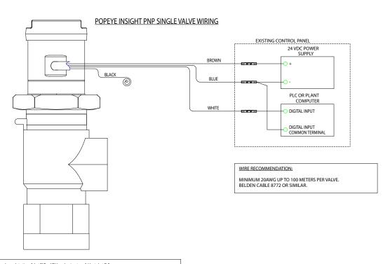
\*Note: Only one signal output can be used at a time. Select PNP or NPN based on inputs available at plant PLC Consult a controls specialist or PLC manufacturer to determine which input is available.
