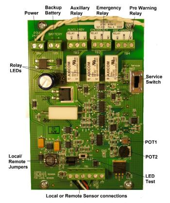
FRONT PANEL MOUNTED CIRCUIT BOARD
