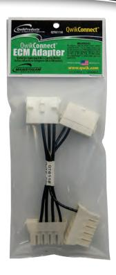
This adapter has two plugs on the one end to receive the plugs that were intended for an ECM 2.3 / Eon motor (J1 for Power, J2 for Communications). The signals from J1 and J2 are wired to the appropriate plugs for the Evergreen® Motor (P1 for Power, P2 for Communications).
