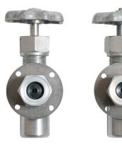
Gauge set assembly is of all steel construction and all parts are zinc plated. Gauge valves have safety ball seats which automatically shut off liquid in case of glass breakage. Valve stems are packed with composition packing rings, providing a leak-proof, long life seal.
