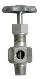
Purge valves are made of all steel and all parts are zinc plated. They are used for purging purposes and are supplied with male and female thread combinations. They are equipped with round malleable handles. This valve can be used for gauge mounting, as an oil drain, or any place where a small shut-off valve can be used.
