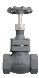
Bolted bonnet shut-off valves in a globe or angle design to work with pipe sizes from 1 ¼" to 2". This sturdy valve body is made from cast iron and is pressure tested for leakage after assembly.
