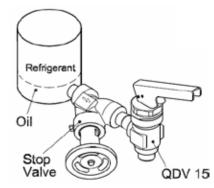
\* QDV valve train includes QDV 15 with 1/2 in. FPT x 1/2 in. FPT connections and an SVA-ST 15 globe stop valve with hand wheel and 1/2 in. socket-weld inlet x 1/2 in. male NPT outlet connections for quick on site mounting.
