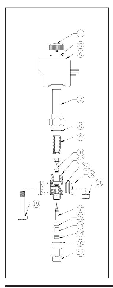
through the valve. When de-energized, the spring in the #9 Plunger-Needle-Assembly forces the valve closed.
