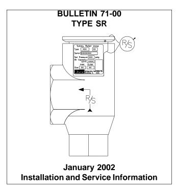
stainless steel, and a PTFE disc prevent sticking due to corrosion or cold welding and assure valve opening at the set pressure long after installation. They are not suitable for corrosive ambient atmospheres such as chlorine, etc. Connection sizes are 1/2" FPT inlet with 3/4" or 1" FPT outlet. A 3/4" inlet with 1" FPT outlet is also available.
