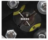
Select sizes on underside of dies to match tubing
