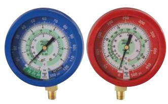
Gauges are completely filled with glycerin for maximum protection from pulsation. Large 3-1/2" (90 mm) diameter gauge with refrigerants color-coded on the dials in bold numbers. Offset stem fits all major manifold brands.
