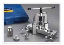
60455 large-size swages and flares for  $3/4\ensuremath{^{\text{H}}},\,7/8\ensuremath{^{\text{H}}}$  and 1-1/8 $\ensuremath{^{\text{H}}}$  O.D. tubing
