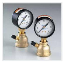
Easy-to-read gauge to test system pressure for leaks in new installations. Pressure drop indicates leakage. 0-30 gauge is in 1/4 lb. increments and 0-15 gauge is in 1/5 lb. increments. Brass threaded bell for leak tight connection.
