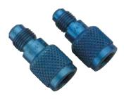
Liquid charging is recommended when charging blends into refrigeration and air conditioning systems. A liquid charging adapter is necessary for safe and fast liquid (saturated vapor) charging through the low pressure side of a system. The YELLOW JACKET liquid charging adapter connects to the cylinder valve or refrigerant tank.
