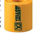
The YELLOW JACKET® Solenoid Valve Service Magnet is the quickest and easiest way to manually operate solenoid valves. It works by magnetically lifting the stem assembly and plunger to actuate the valve during service.
