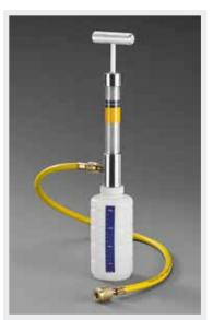
Self-contained injection system for inducing up to 16 oz. of universal AC/R dye into the largest systems. Add to the lo-side. Easily works on all system pressures to 300 psi, .35 oz. per stroke. Hose included with SealRight end.
