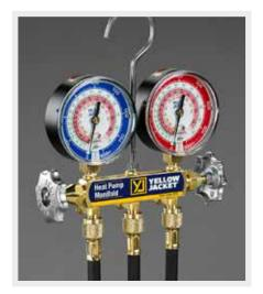
The YELLOW JACKET® Heat Pump Manifold features two 800 psi gauges to read all heat pump pressure conditions. Traditional lo-side manifold gauges can be susceptible to damage when heat pumps go into heating mode. Because the lo-side gauge of the YELLOW JACKET Heat Pump Manifold is also designed for pressures up to 800 psi, it can read the pressure whether the pump is in heating mode, cooling mode or transition.
