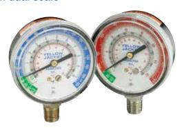
Ammonia gauges are designed for use on manifolds and as permanent gauges on any system or equipment charged with ammonia. The Bourdon tube is made of 316 stainless. The dials show dual temperature and pressure scales. All gauges are equipped with restrictors to protect the gauges against pulsating pressure.
